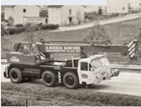
Bestseller from Ehingen (Germany): the AUK 40T-60 with its 24-metre telescopic boom and fully hydraulic crane drive.
