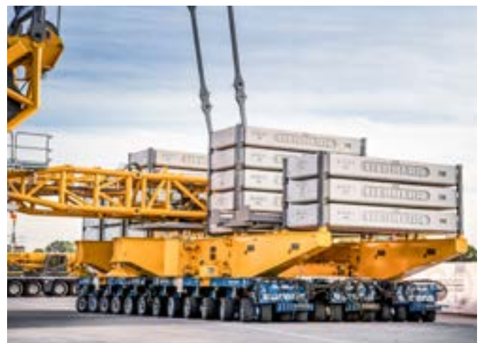
36 SPMT axles are used as ballast wagons for the LR 12500-1.0.
