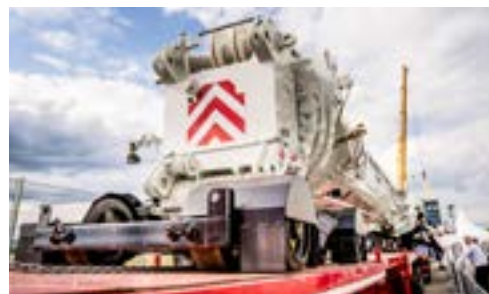
The trolley with chain drive pushes the boom towards the crane for assembly.
