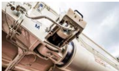
The boom is bolted together quickly and easily using the remote control.
