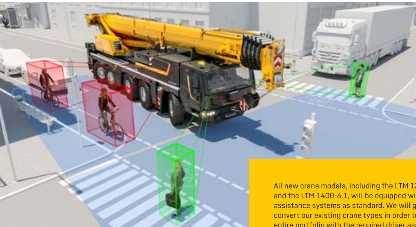
The driver assistance systems scan the surroundings and warn the crane driver to prevent accidents.
