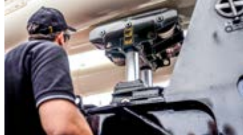
A device is attached to the rear of the crane, which raises the boom.
