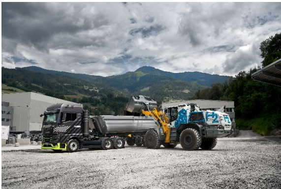
liebherr-L566-H2-wheel-loader-Bischofshofen.jpg The Liebherr plant in Bischofshofen presented the first large wheel loader with a hydrogen engine.
