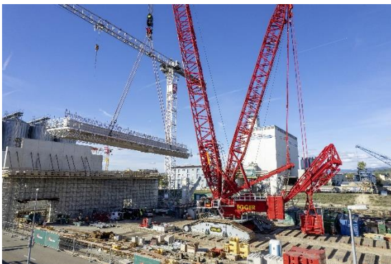
liebherr-lr-11000-egger-5.jpg The V-frame allows the ballast radius to be reduced quickly and easily on confined construction sites.
