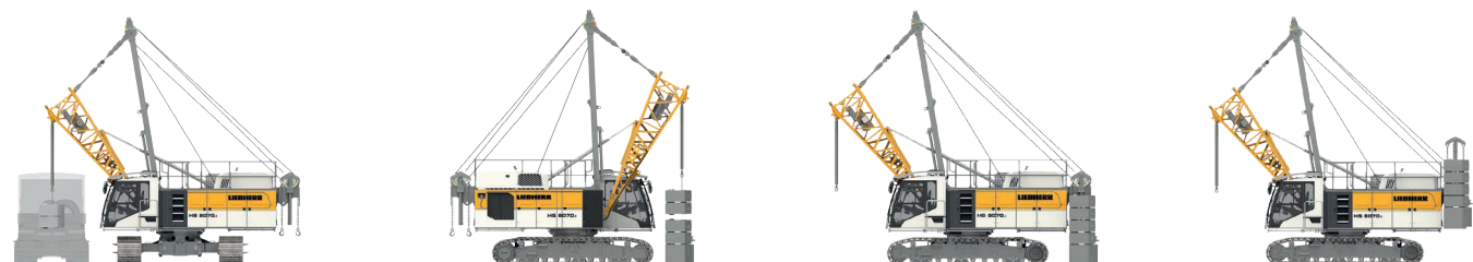
Unloading and assembly of rear counterweight
