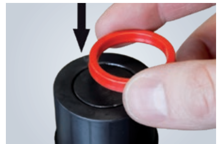
3. Press together new sealing washer and place on the sealing disc with the open end facing downwards.
