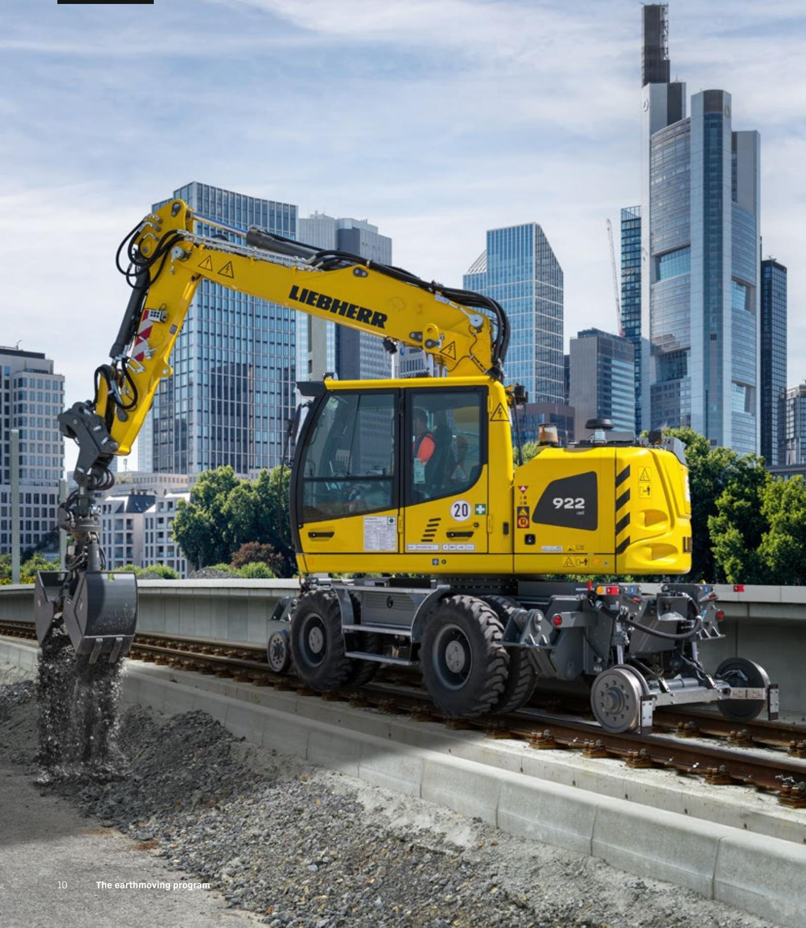
Liebherr has been developing rail-road excavators since 1967 and – as an OEM manufacturer – is the world market leader in this field. These machines are adapted to country-specific specifications (e.g. track width) and therefore comply with local conditions and safety regulations. Our rail excavators can be used either on the road or on railway tracks.
