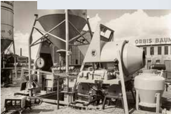
The first reverse drum mixer – still a pre-series model here – becomes a bestseller.
