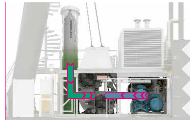
Discharging of the accumulator
