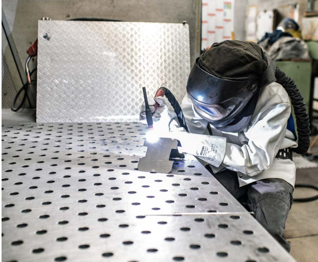
Using the tungsten inert gas welding process, an apprentice manufactures an aluminum sheet metal bracket
