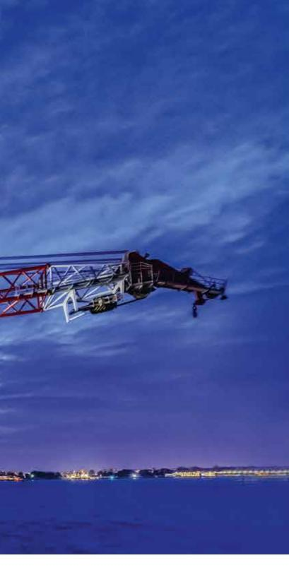
The board offshore crane is available in various sizes and different lifting capacities ranging from 25t up to 1,200t. The boom length can be specified and extended to more than 100 m for some models.
