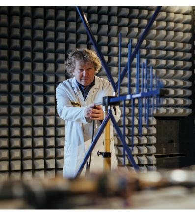
Our test center examines electromagnetic compatibility (EMC) for you in accordance with all common standards in the aviation, automotive, railway and commercial industry sectors (RTCA/DO-160, MIL-STD, CISPR 16/25/32, DIN EN 61000 amongst others).
