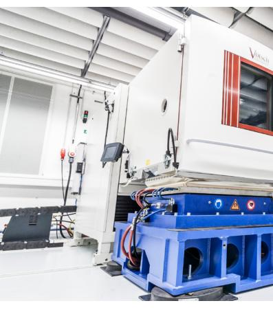
The constantly increasing demands on the mechanical reliability of electronic devices necessitate extensive vibration and shock tests. The Liebherr test laboratory has two electrodynamic vibration test systems at your disposal, which you can use both for development purposes and for certifications.
