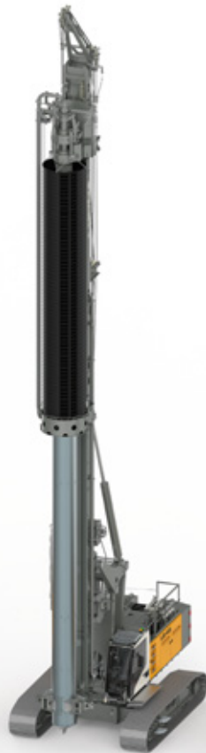
Double rotary drilling
