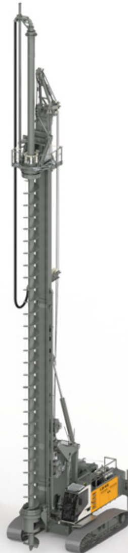
Continuous flight auger drilling with Kelly extension
