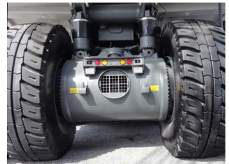
Service door on axle box for inspections
